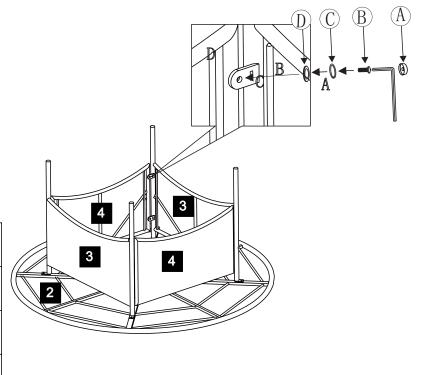
Remember to fully tighten all bolts before turning over. next
