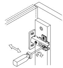
Turn Inner screw to move door in or out
