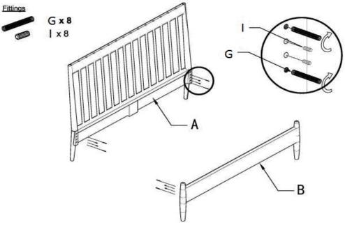
STEP 2. Making sure the holes in the side rails, C, are facing upwards, AND you have the Left and Right rails, (see page 4) on the corret sides, locate these side rails onto the protruding threads on the headboard and footboard. As you do this, slide a half moon washer onto the thread when it comes through into the circular hole in the side of the rail, then screw on one of the 8 nuts FINGERTIGHT ONLY. Repeat with the other 3 corners then TIGHTEN FIRMLYWHEN ALL FOUR CORNERSARESECURED
