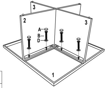
Remember to fully tighten all bolts before turning over.
